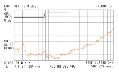
Prescan from Compact 3 Meter Chamber, no Measurable signals on 3 Meter OATS.
