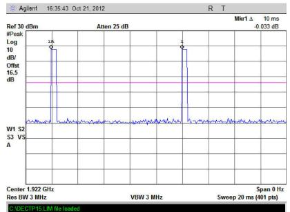
Result: Compliant, plot is used to demonstrate this is a 10 mS or shorter system. This requirement is covered by the results of the LIC test performed in Section 6.11.7 of this report.
