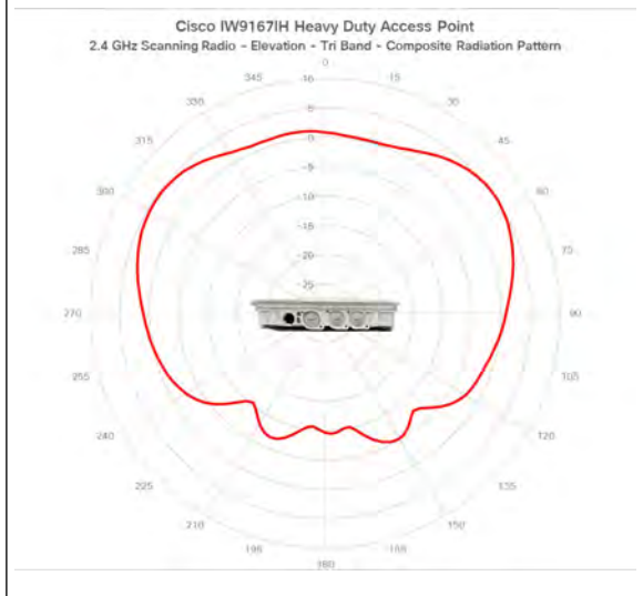
Figure 14: IW9167IH - Scanning Radio-Tri Band Composite Radiation Pattern (2.4-GHz Elevation)
