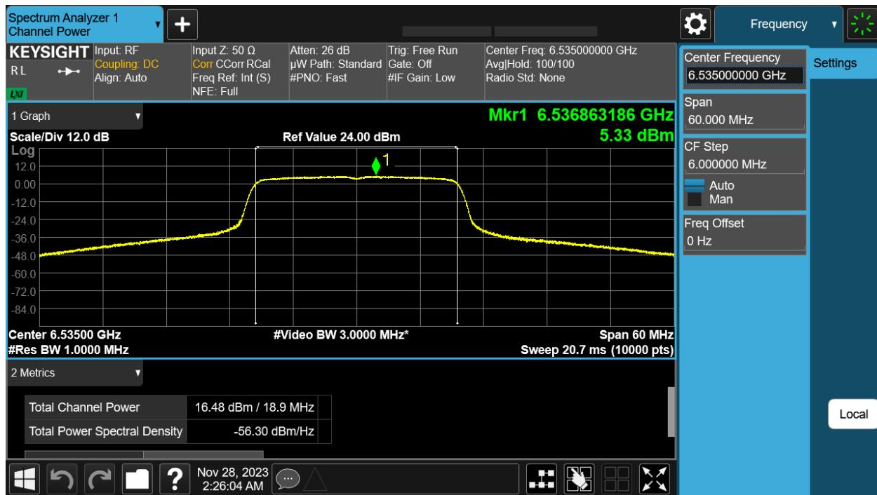
6535 MHz: HE20 Beam Forming, M0 to M11 1ss – Antenna B
