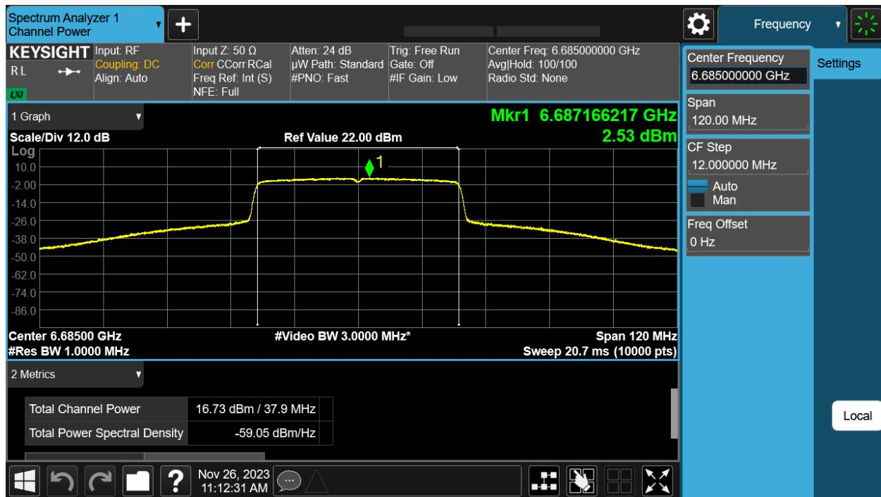
6685 MHz: HE40 Beam Forming, M0 to M11 1ss – Antenna B
