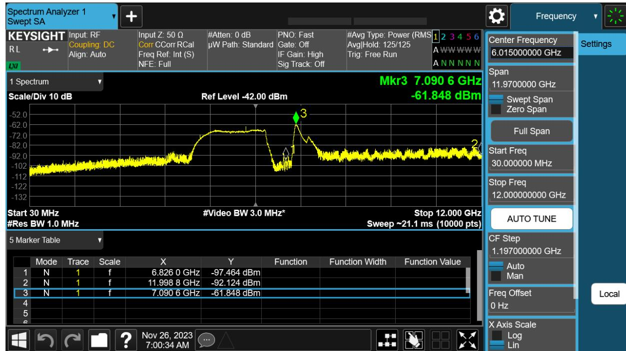
**Conducted Spurious emissions Peak – Antenna gain 7dBi – 20MHz BW.**
