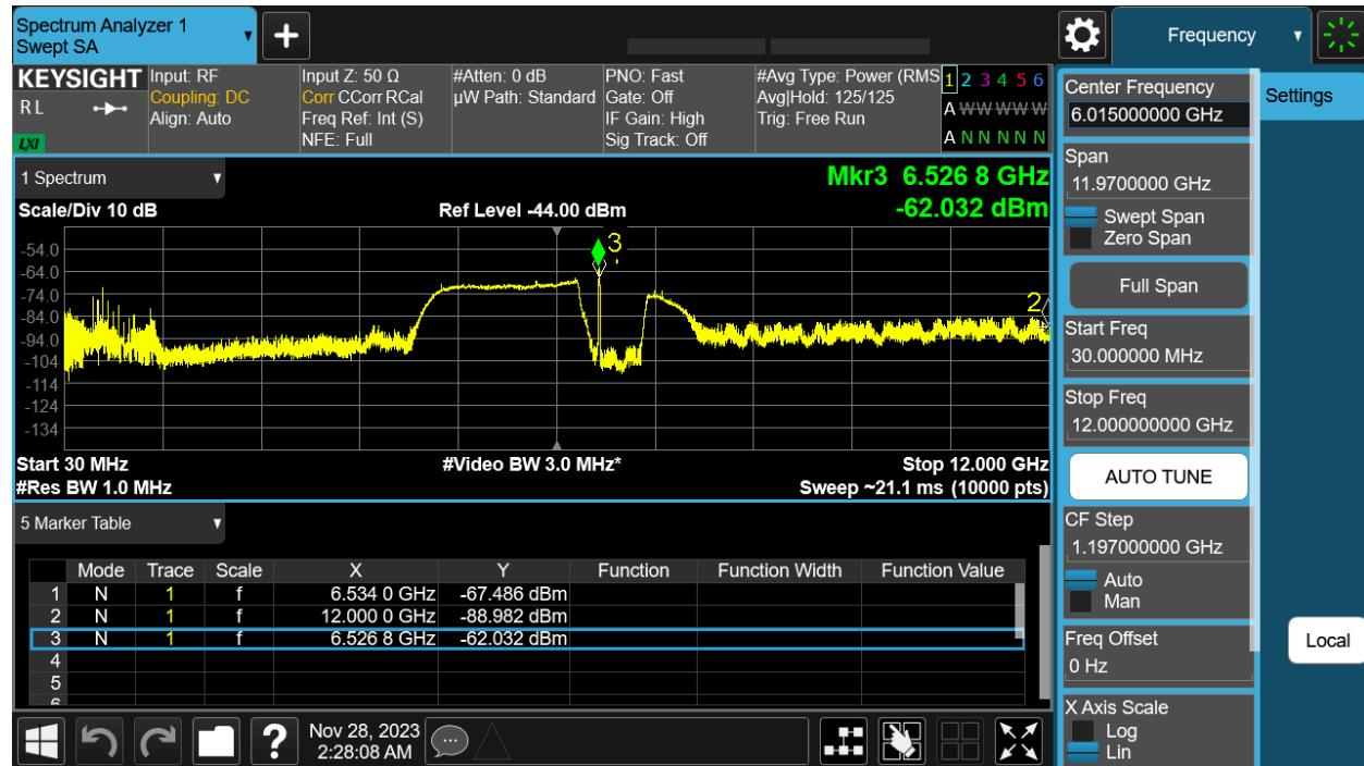
6535 MHz: HE20 Beam Forming, M0 to M11 1ss – Antenna B
