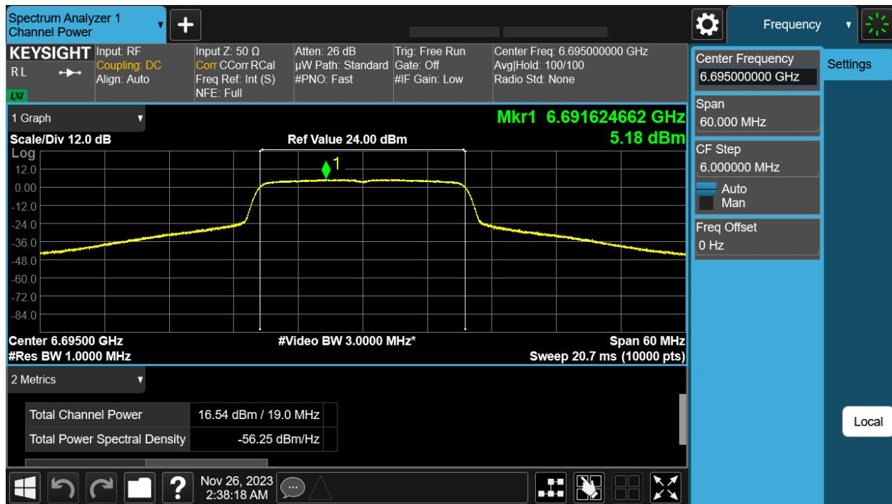
6695 MHz: HE20 Beam Forming, M0 to M11 1ss – Antenna B
