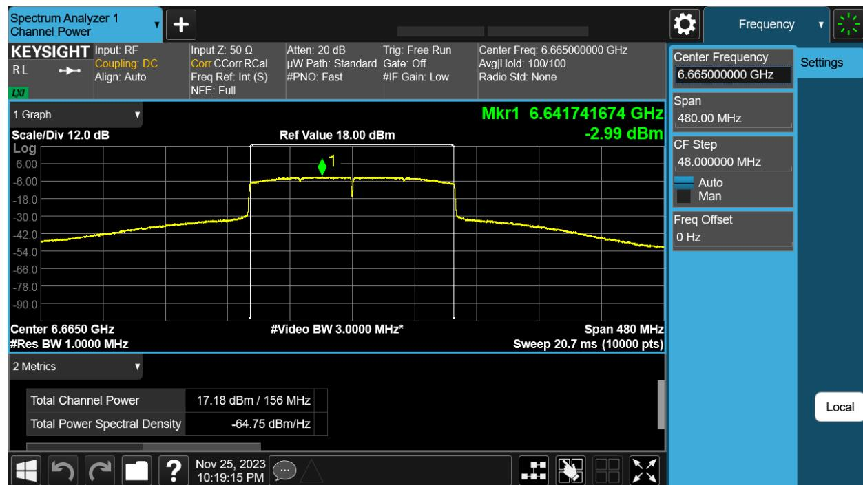
6665 MHz: HE160 Beam Forming, M0 to M11 1ss – Antenna B
