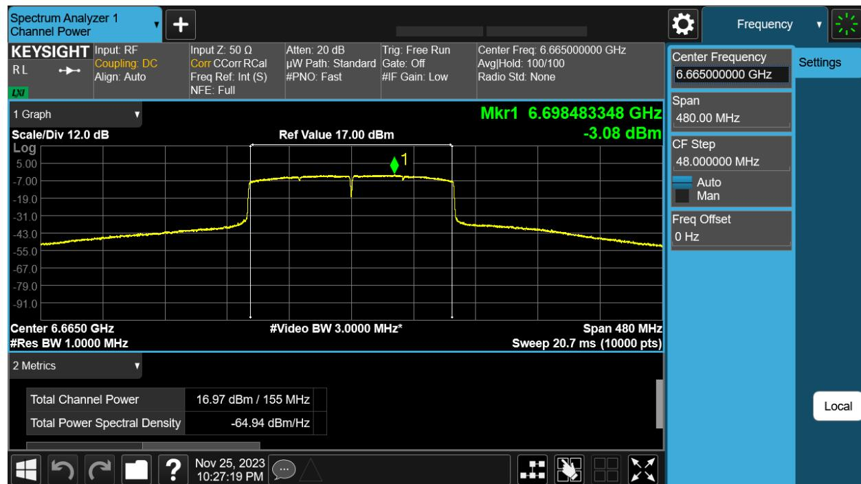
**Maximum Transmit Power > 30° - Antenna gain 7dBi (-4dBi) – 20MHz.**
