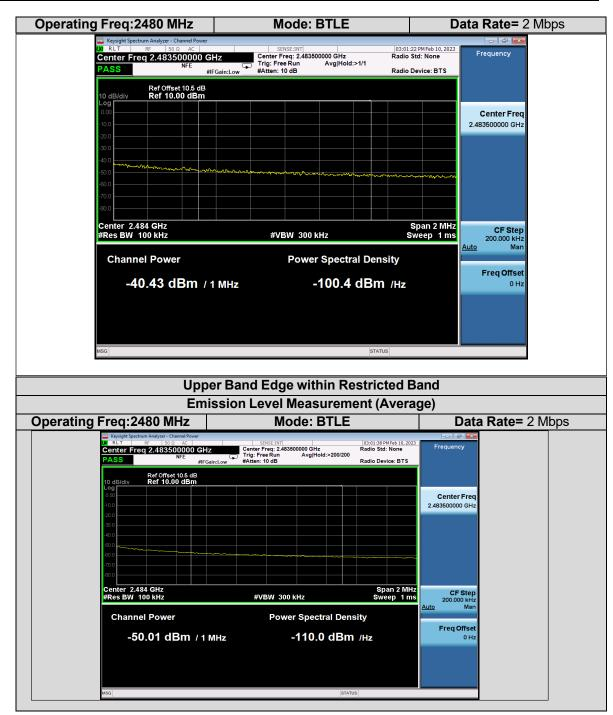
Note: Upper bandedge power integration was performed with the integration band centered on the bandedge instead of starting from the bandedge. As this results in a measurement being performed closer to the fundamental with higher amplitude, worst-case compliance is shown
