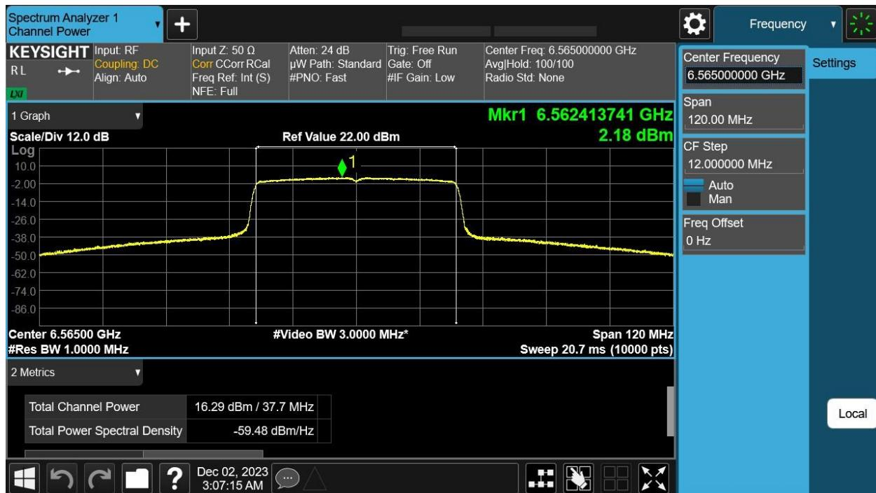
6565 MHz: HE40 Beam Forming, M0 to M11 1ss – Antenna B
