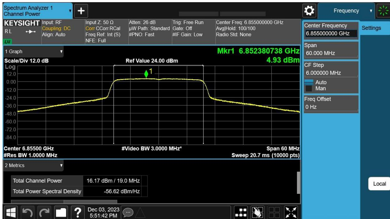
6855 MHz: HE20 Beam Forming, M0 to M11 1ss – Antenna B
