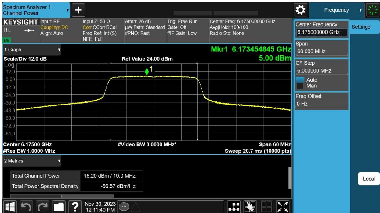
6415 MHz: HE20 Beam Forming, M0 to M11 1ss – Antenna A
