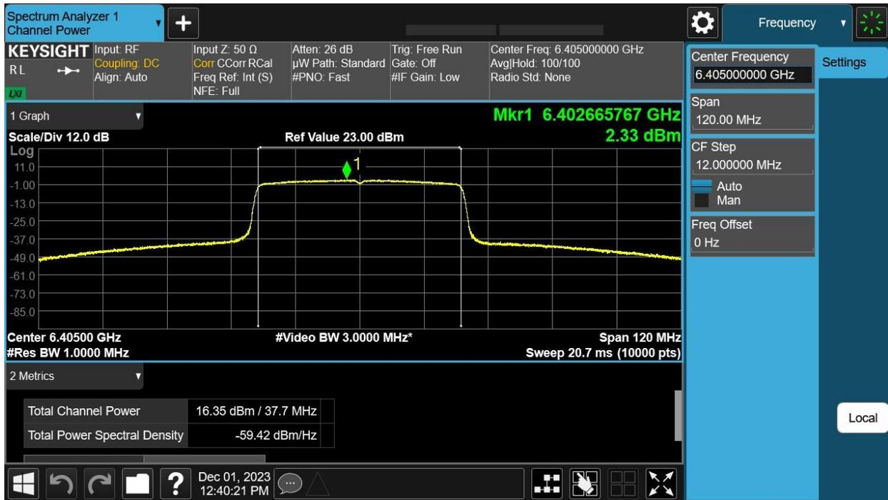
6405 MHz: HE40 Beam Forming, M0 to M11 1ss – Antenna B
