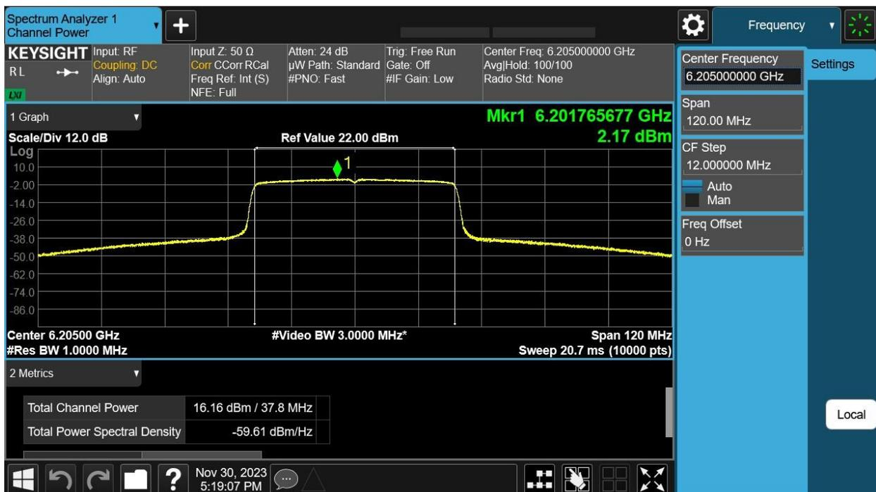
6405 MHz: HE40 Beam Forming, M0 to M11 1ss – Antenna A
