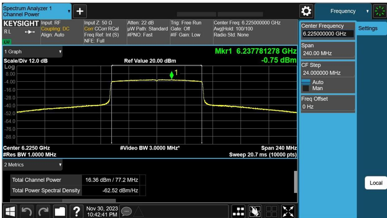
6385 MHz: HE80 Beam Forming, M0 to M11 1ss – Antenna A
