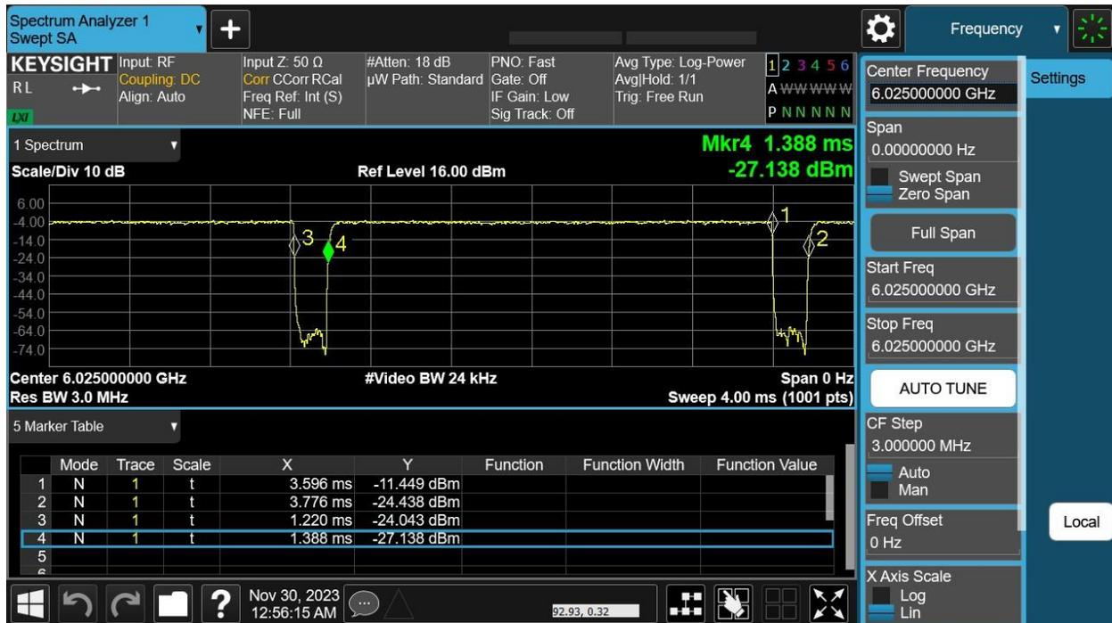
**A.2: 99% and 26dB Bandwidth****99% and 26dB Bandwidth Test Requirement**
