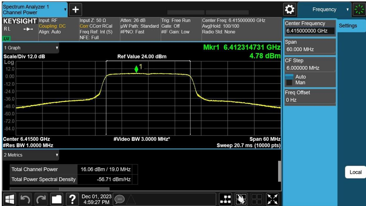
6415 MHz: HE20 Beam Forming, M0 to M11 1ss – Antenna B
