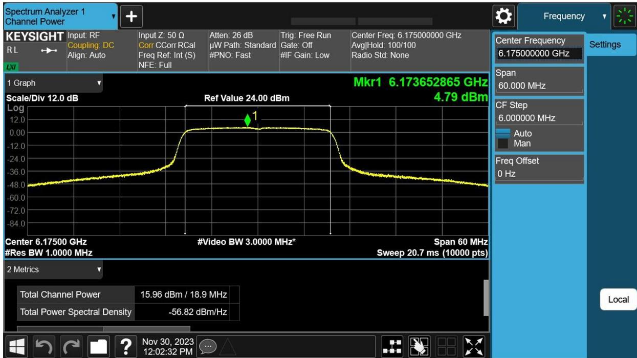
6175 MHz: HE20 Beam Forming, M0 to M11 1ss – Antenna B
