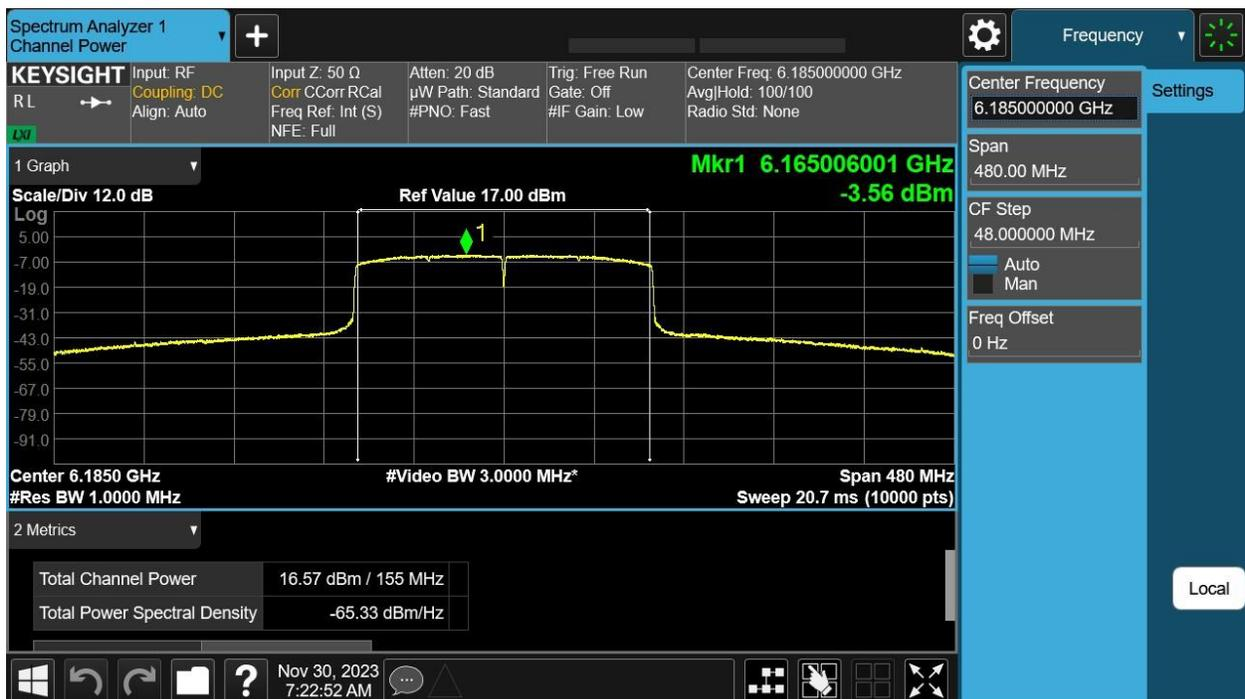
6345 MHz: HE160 Beam Forming, M0 to M11 1ss – Antenna A
