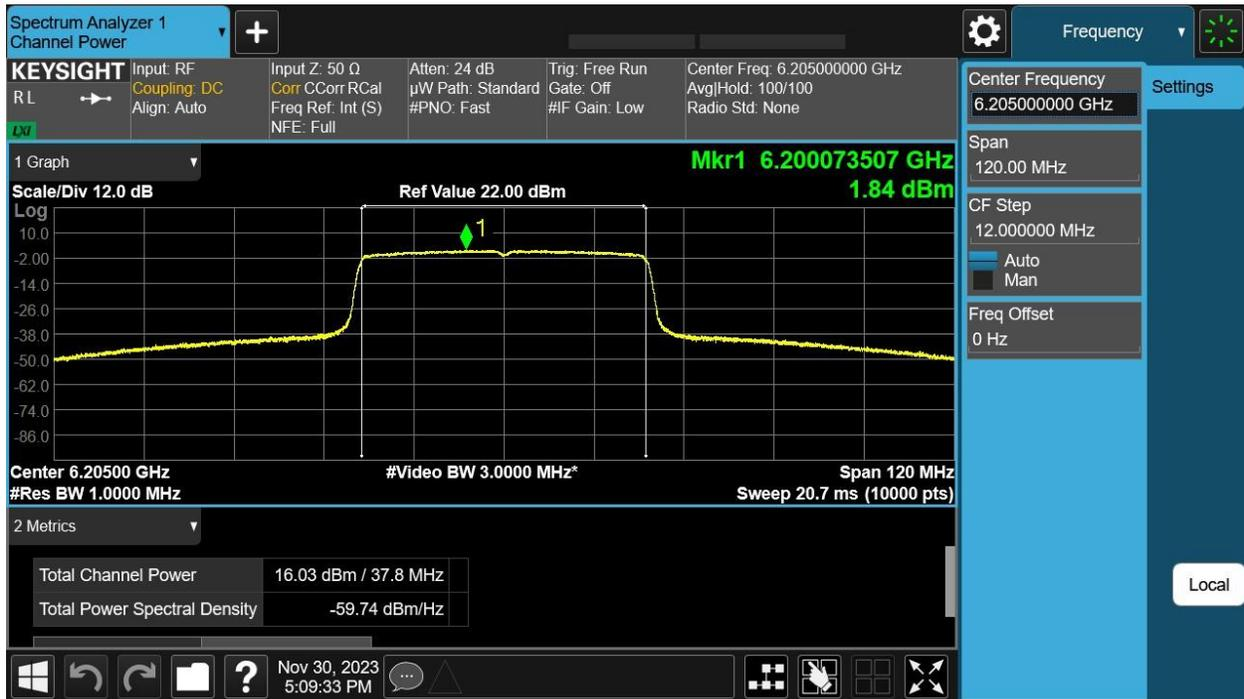
6205 MHz: HE40 Beam Forming, M0 to M11 1ss – Antenna B
