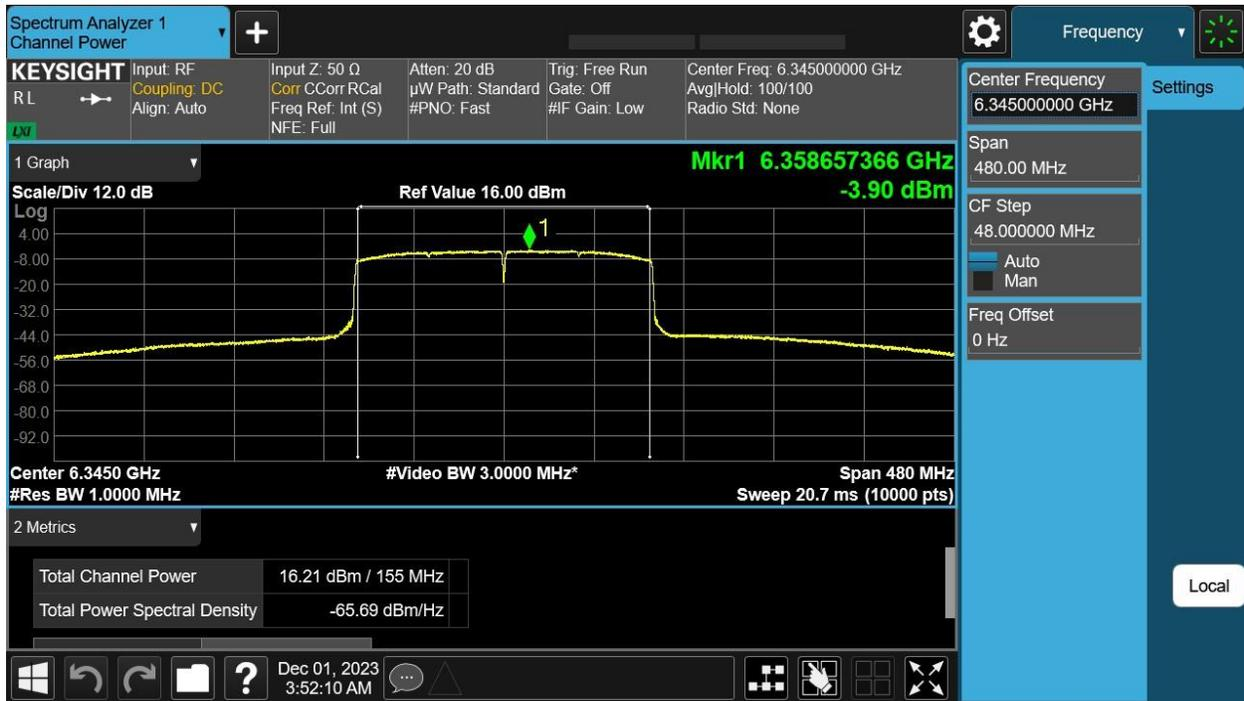
6345 MHz: HE160 Beam Forming, M0 to M11 1ss – Antenna B
