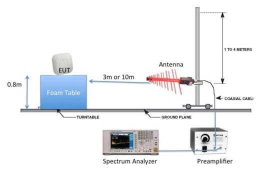
**Note:** The radiated spurious emissions test setup referenced to KDB789033 D02, v02r01, Section II (G)(3)(b)(i)), the EUT antenna ports were terminated with  $50\Omega$  loads.
