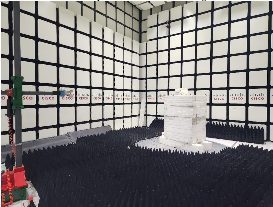
Title: 5GHz Radiated Spurious Emissions Test Configuration 1GHz - 18GHz
