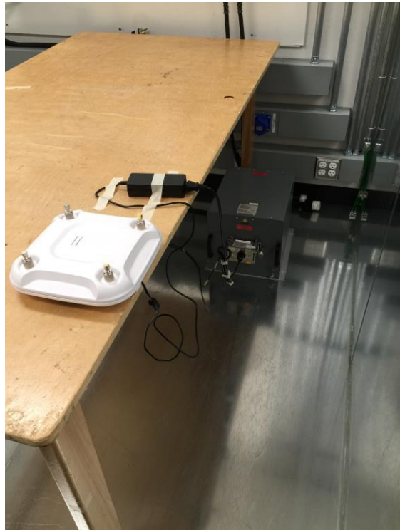
AIR-CAP3702P-B-K9 AC Conducted Emissions setup photo
