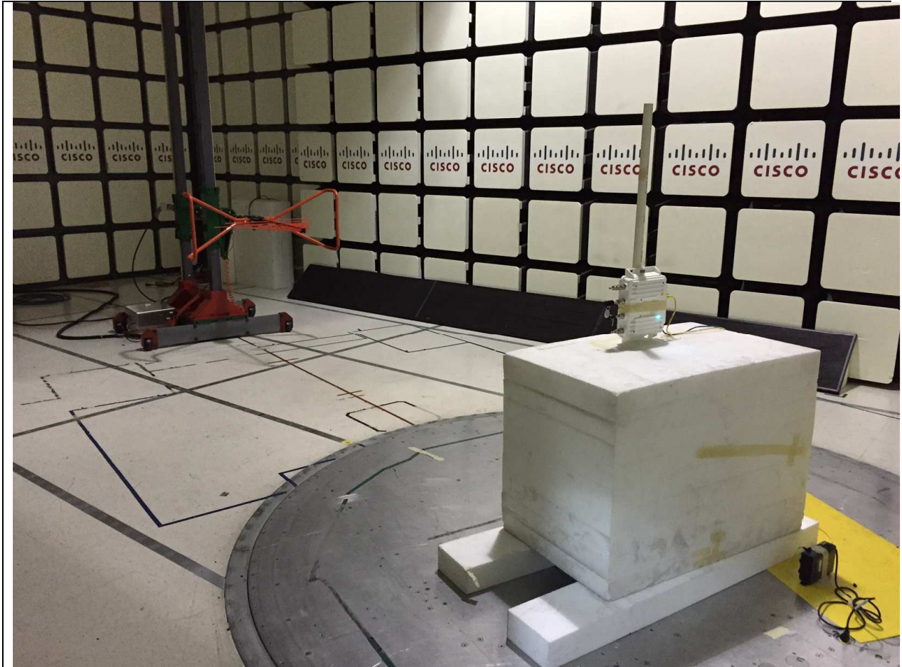
Title: Radiated Spurious Emissions Test Configuration 30M - 1000MHz. EUT is in "Y" orientation. Pol shown = H.
