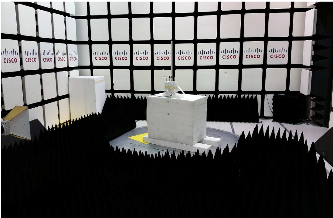
Title: Radiated Spurious Emissions Test Configuration 1G - 18GHz
