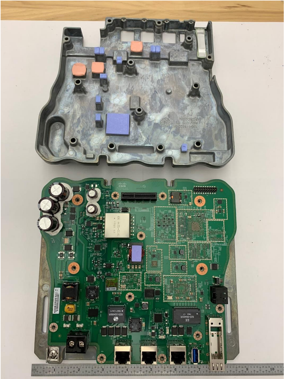
Second casing top cover removed to expose module motherboard top side.
