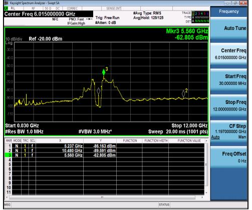
Conducted Spurs Average, 5240 MHz, Non HT20, 6 to 54 Mbps(Antenna internal gain = 4dBi, 5dBi and 6dBi)
