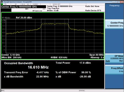
26dB / 99% Bandwidth, 5180 MHz, Non HT20, 6 to 54 Mbps (Antenna internal gain = 4dBi, 5dBi and 6dBi)
