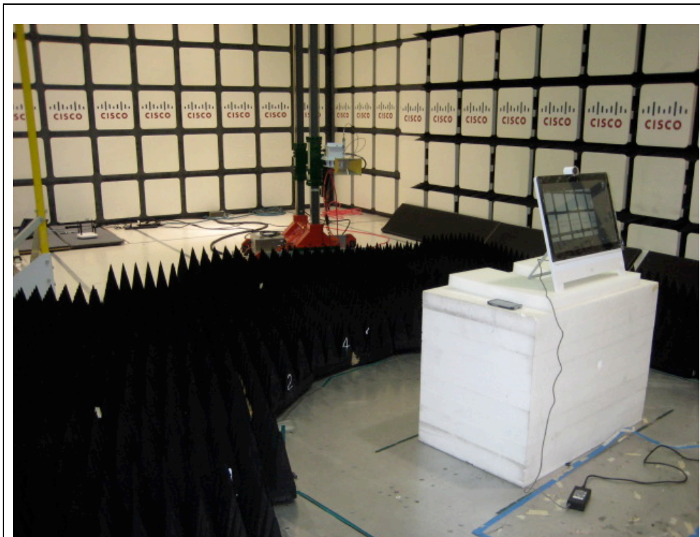
Title: Co-Location Radiated Spurious Emissions 1-18GHz Test Setup
