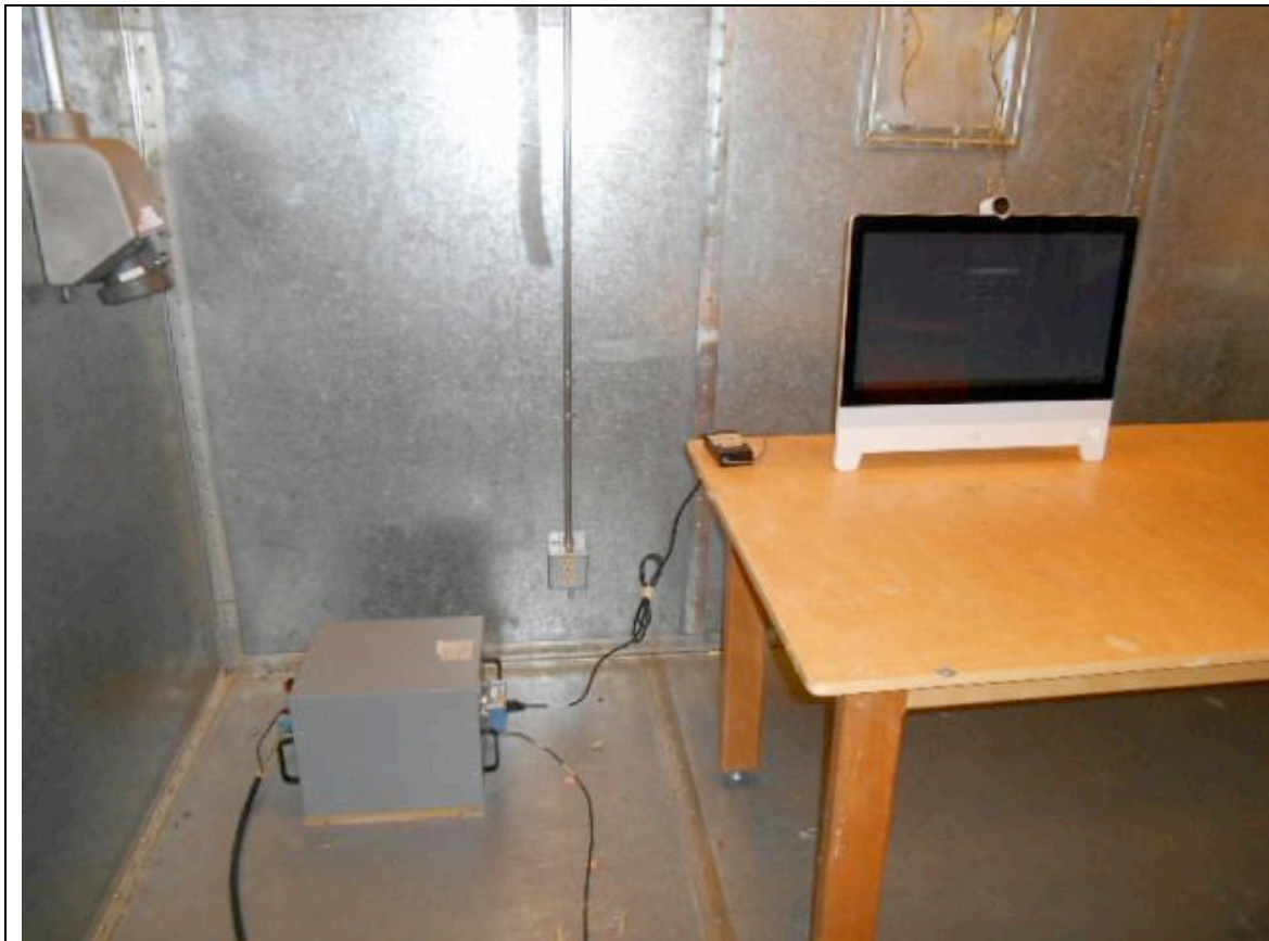
Title: Conducted Emissions Test Configuration
