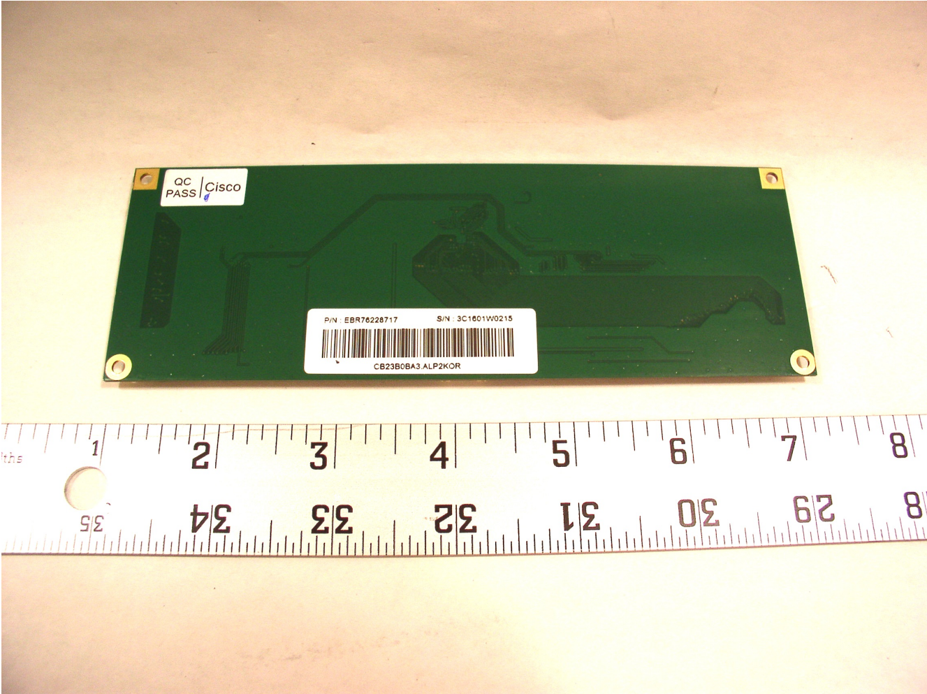
CP-DX80 : Internal PCB touch screen controller (Botom view)
