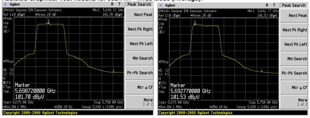
Radiated Graphical Test Results for 802.11A – HT20 Mode (Peak):
