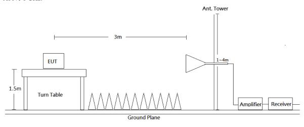
Radiated emission tests were performed in the 3 meters chamber test site, using the setup accordance with the ANSI C63.10-2013. The specification used was the FCC Part 15.209 and FCC 15.407 Limits.
