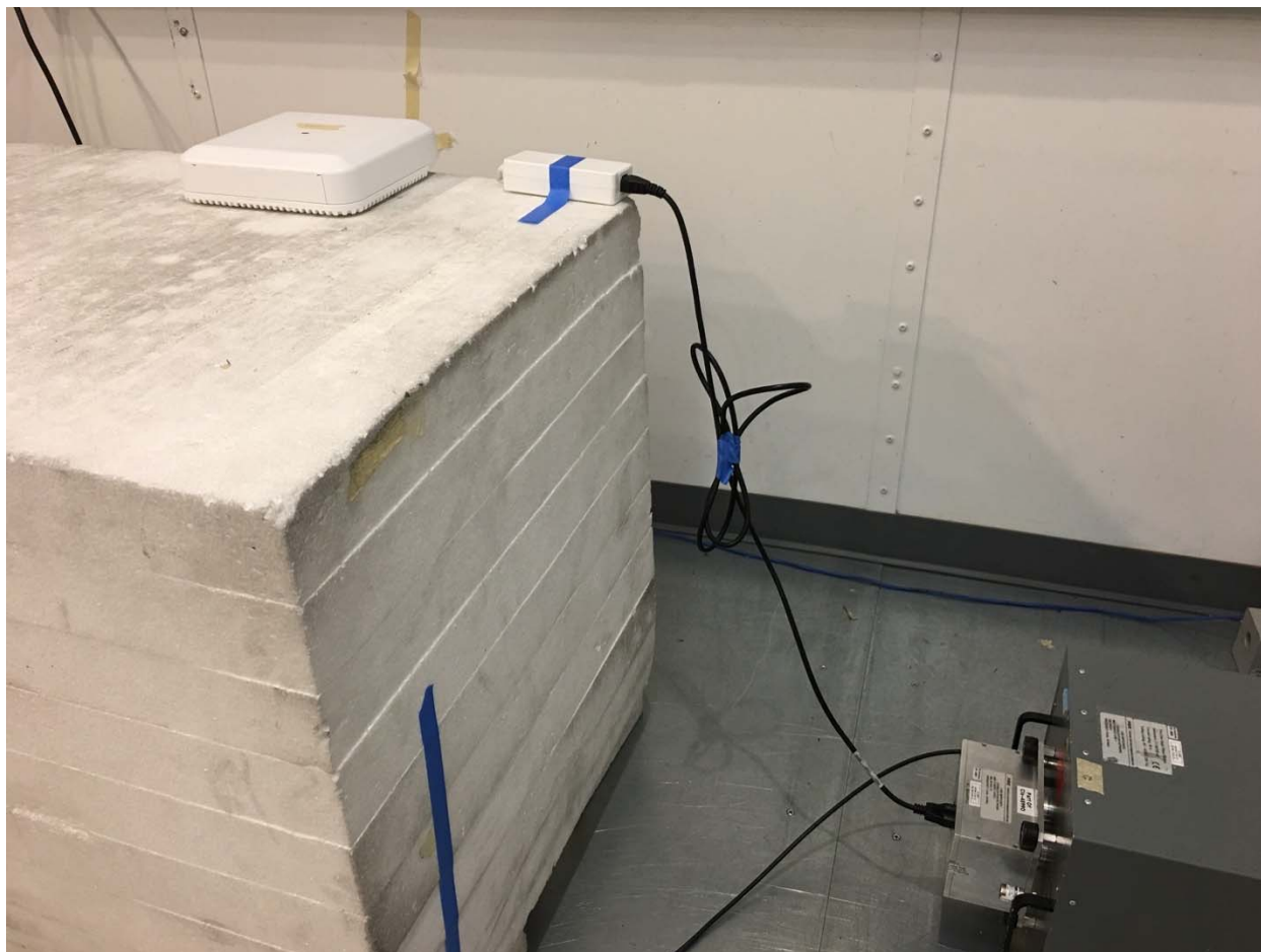
Title: EMC Test Setup, Conducted Emissions on AC lines.
