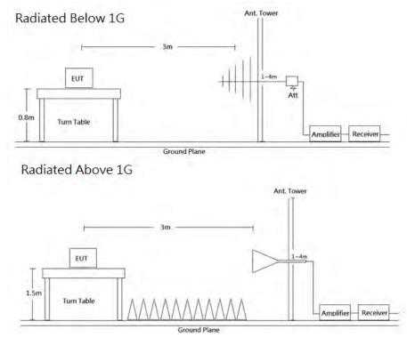
Radiated emission tests were performed in the 3 meters chamber test site, using the setup accordance with the ANSI C63.10-2013. The specification used was the FCC Part 15.209 and FCC 15.407 Limits.
