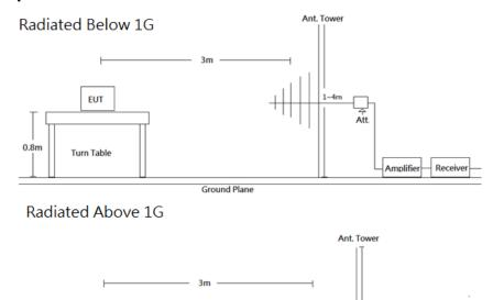
Radiated emission tests were performed in the 3 meters chamber test site, using the setup accordance with the ANSI C63.10-2013. The specification used was the FCC Part 15.209 and FCC 15.407 Limits.
