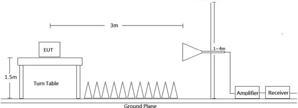
Radiated emission tests were performed in the 3 meters chamber test site, using the setup accordance with the ANSI C63.10-2013. The specification used was the FCC Part 15.209 and FCC 15.247 Limits.
