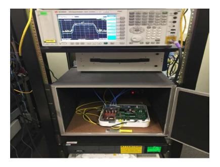
Radiated Test Setup 1-40GHz
