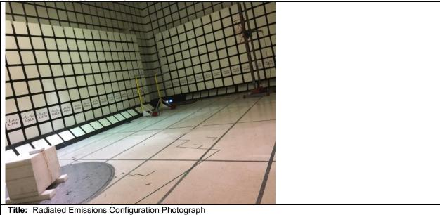
Radiated Test Setup 1-40GHz
