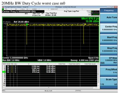
The Duty cycle is 99.2%, no correction is needed for measurements of 20MHz BW.
