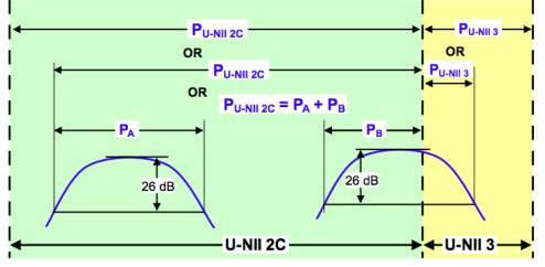
**Conducted output power within a U-NII band:** Integrate over the band, or integrate over a span including the 26 dB EBWs of transmission segments within the band, or integrate over 26 dB EBW of each transmission segment in the band and sum.
