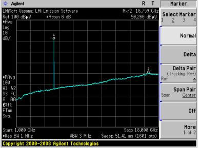
Average Radiated Transmitter Spurs, 5500 MHz, 6 to 54 Mbps
