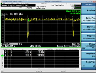
The Duty cycle of 80MHz BW is 97.3%, a 0.2dB CF is added to measurements.
