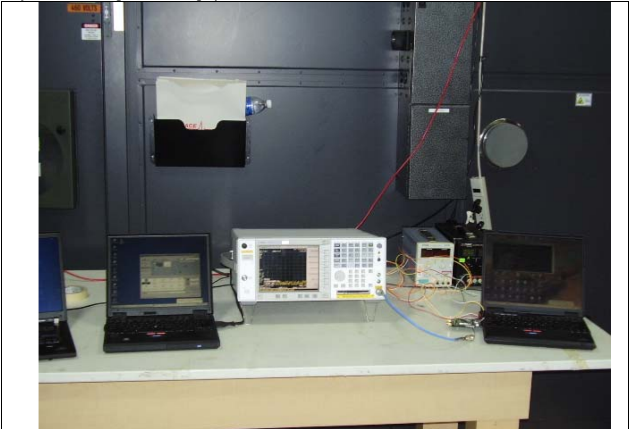
Title: Conducted 26db bandwidth test setup
