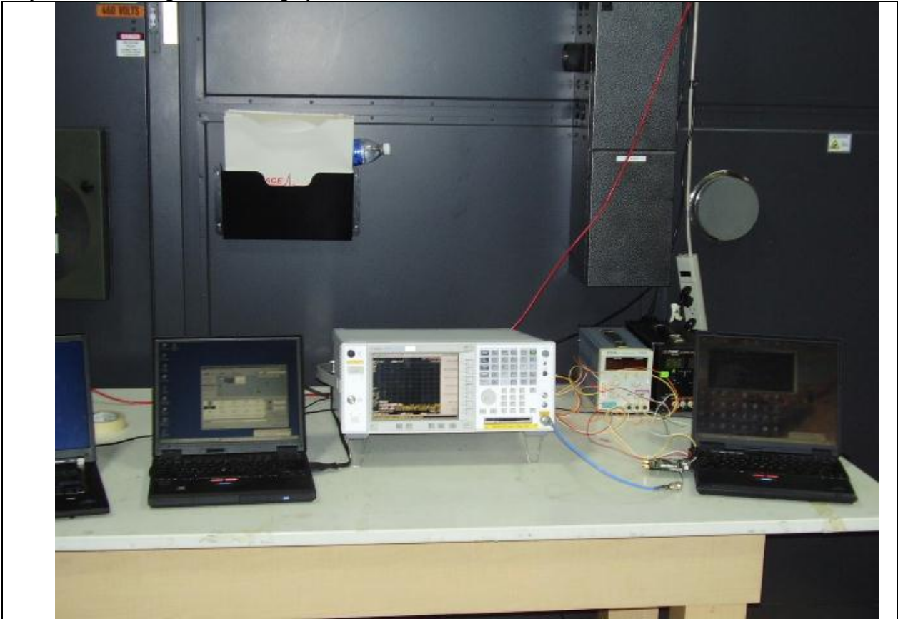
Title: Conducted measurement test setup
