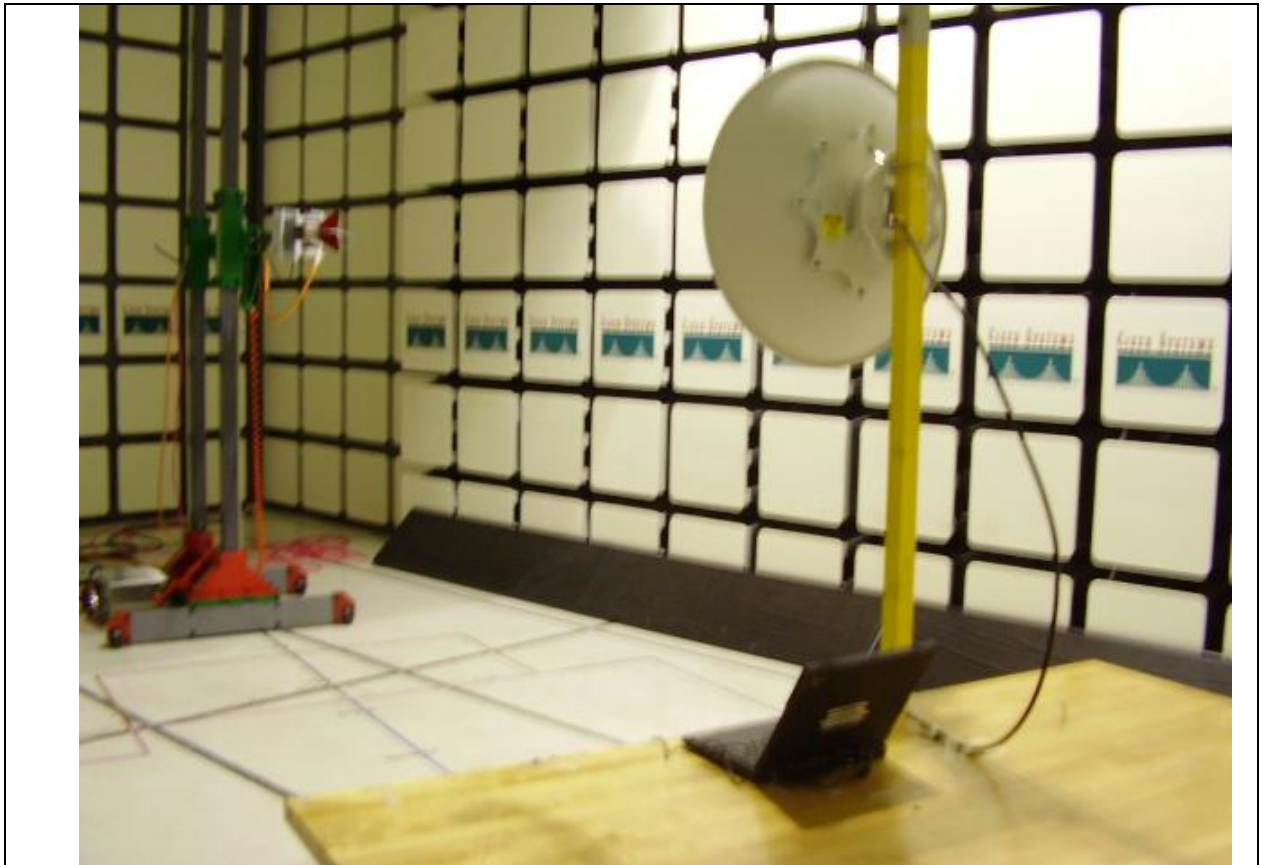
Title: Radiated emissions test setup
