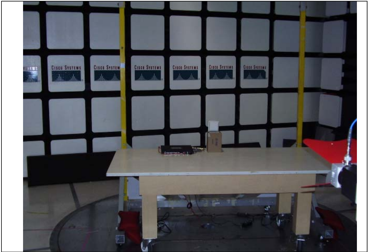
Title: Radiated emissions test setup
