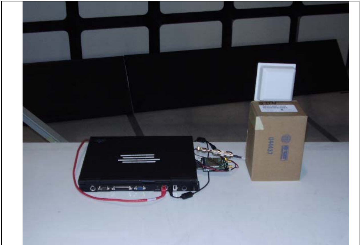
Title: Radiated emissions test setup
