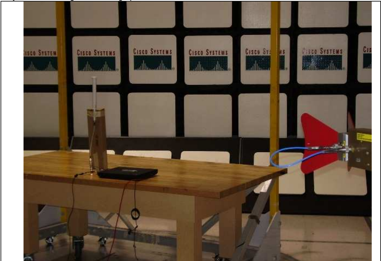
Title: Bandedge test for 7.5dbi Omni test setup
