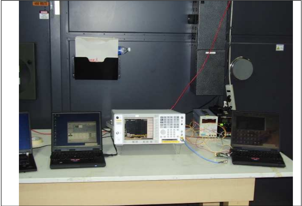
Title: Conducted measurement test setup
