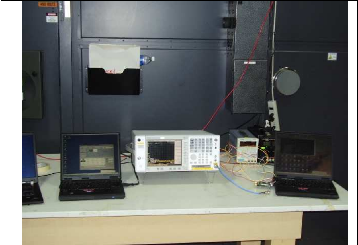
Title: Conducted measurement test setup
