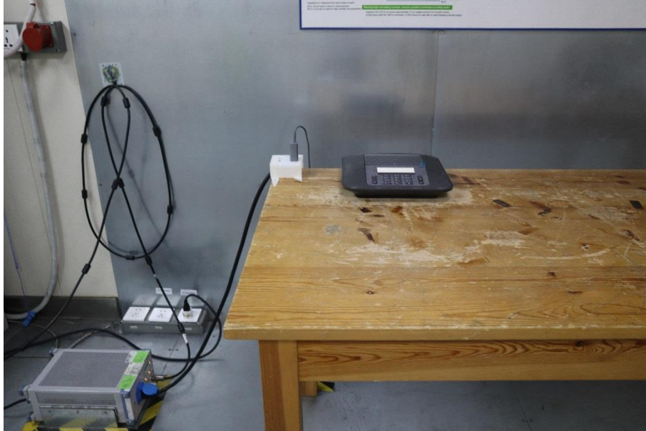
Radiated Spurious Emission ( Below 1GHz )
