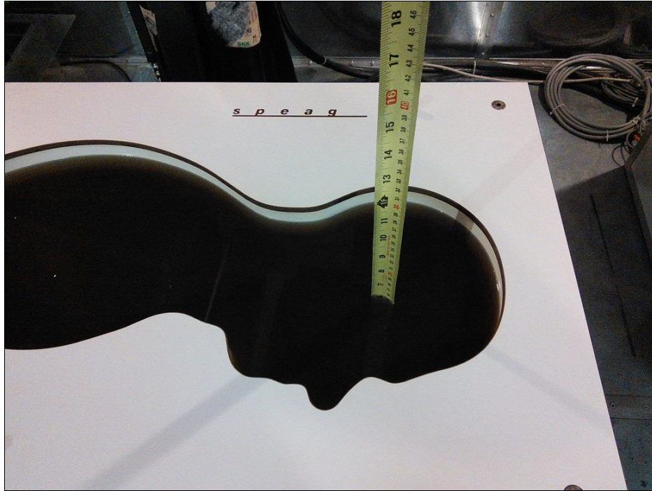
Figure 22: 5GHz head tissue simulating fluid.
