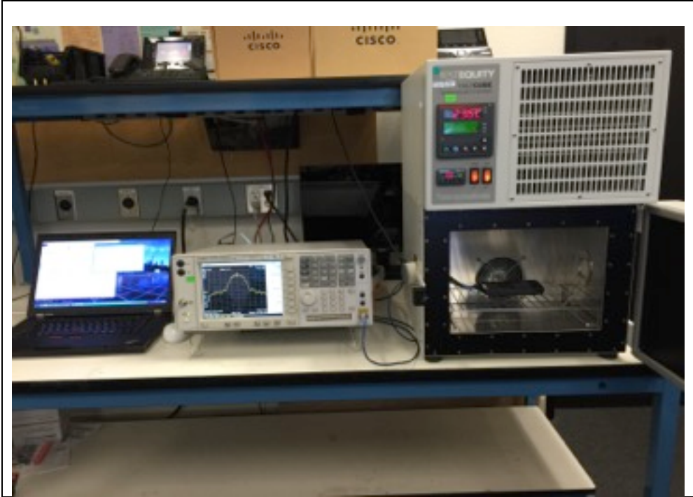
Title: Temperature / Frequency Stability Test Set Up
