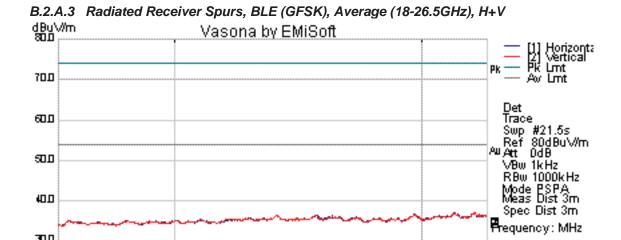
Radiated Emissions Template: B 18-26.5GHz Formal(3m)
