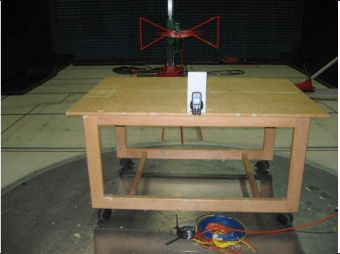
Title: Radiated Spurious Emissions Test Configuraiton for 30M - 1000MHz
