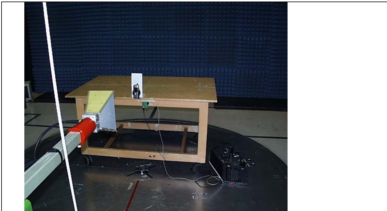
Title: Radiated Spurious Emissions Test Configuraiton at 1m (Front View)
