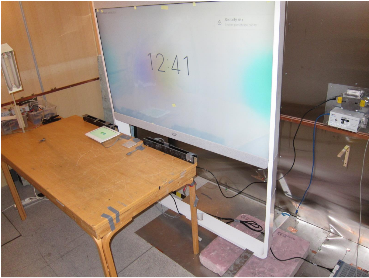
Power line Conducted Emissions Test
