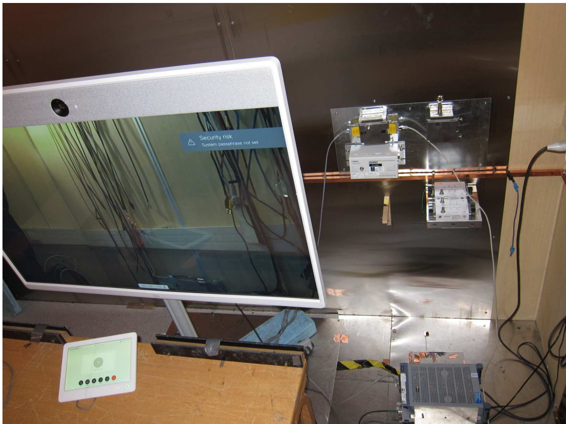
Power line Conducted Emissions Test
