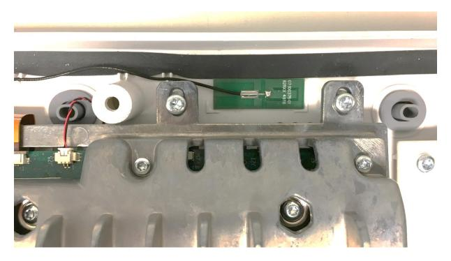
Antenna in near top center of the product. The rear side of the antenna PCB is only glue, no PCB traces.
