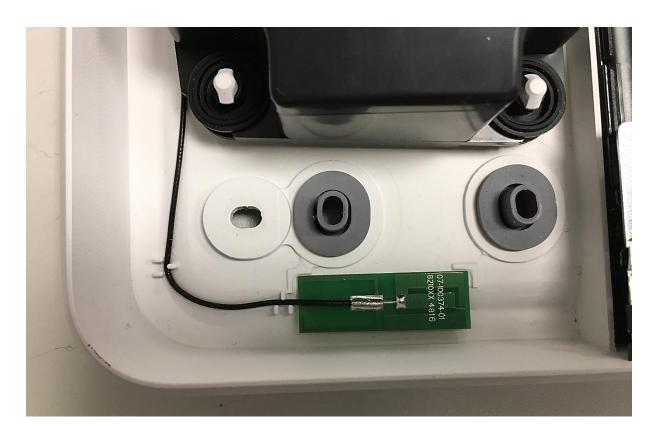
Antenna in the corner of the product. Rear side of the antenna PCB is only glue, no PCB traces.
