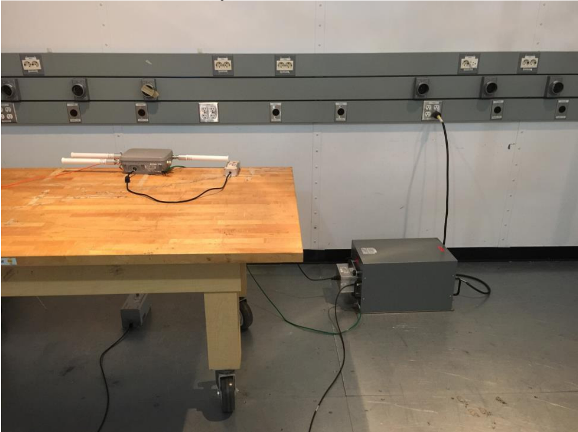
AC Mains Conducted Emissions setup
