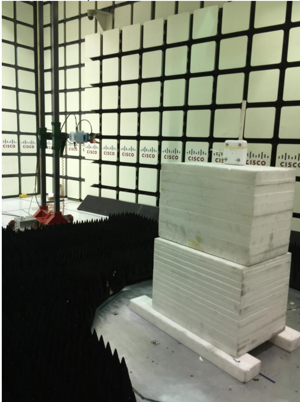
Radiated Emissions setup above 1GHz
