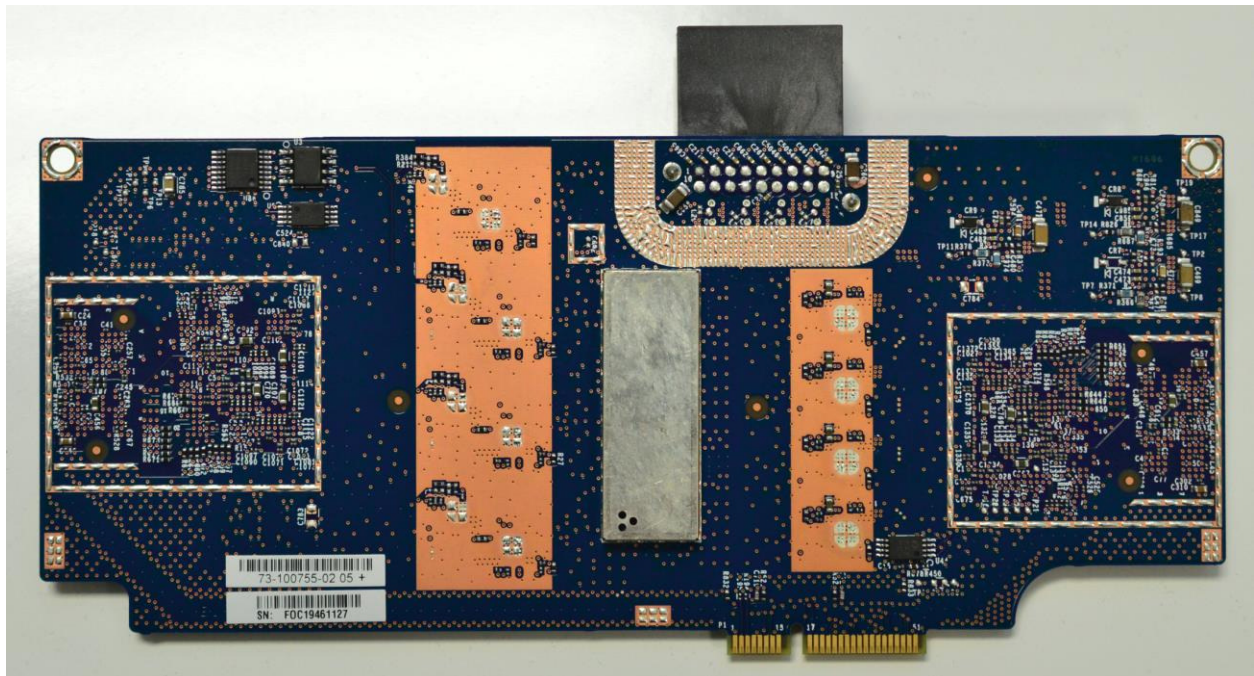
Bottom Side RF Board Without Shield
