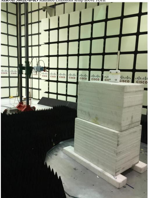
AIR-AP3802E-B-K9 Radiated Emissions setup above 1GHz
