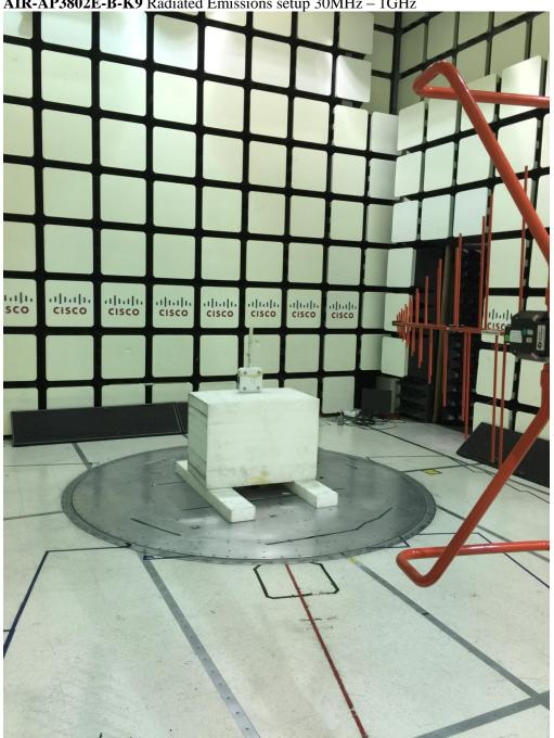
AIR-AP3802E-B-K9 Radiated Emissions setup 30MHz – 1GHz
