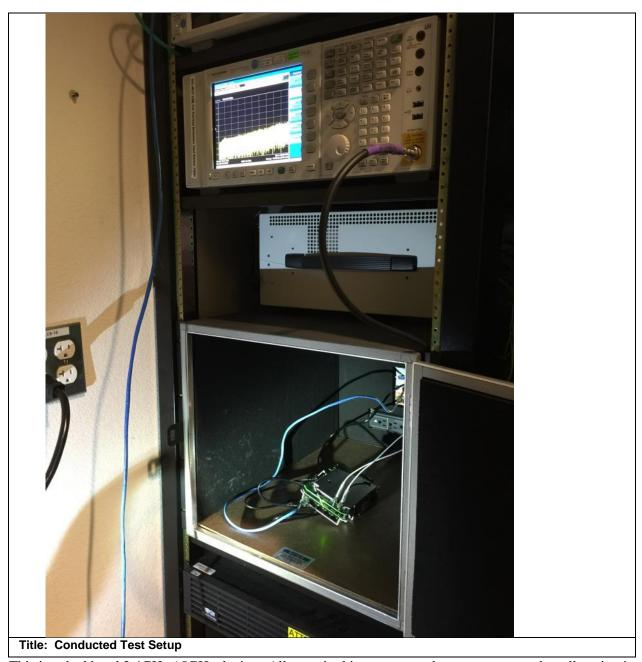
This is a dual band 2.4GHz / 5GHz device. All ports in this test set up photo are connected as all testing is automated. Section 2.6 of this test report given an overview of the different Tx antenna combinations used by this device.
