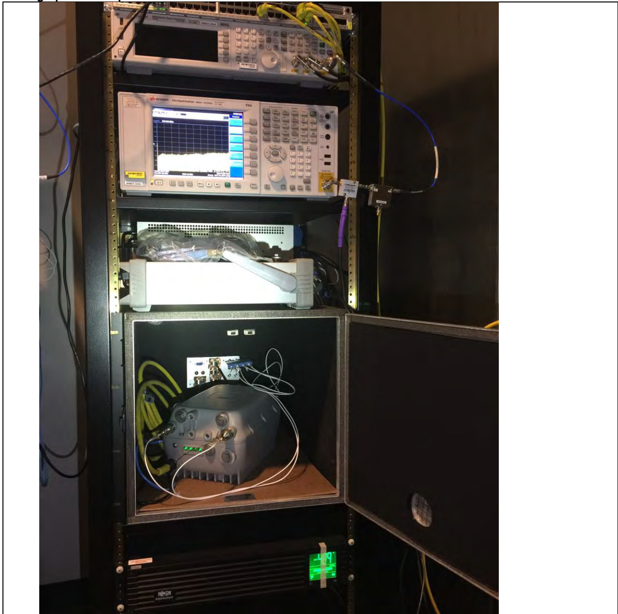
This is a dual band 2.4GHz / 5GHz device. All ports in this test set up photo are connected as all testing is automated. Section 2.6 of this test report given an overview of the different Tx antenna combinations used by this device.
