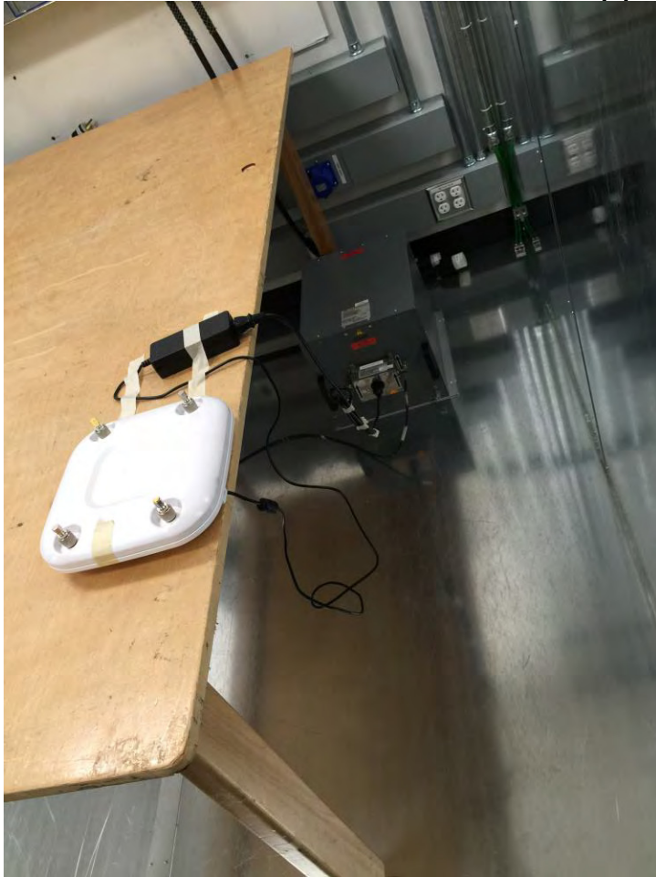
AIR-CAP2702E-B-K9 AC Conducted Emissions setup photo
