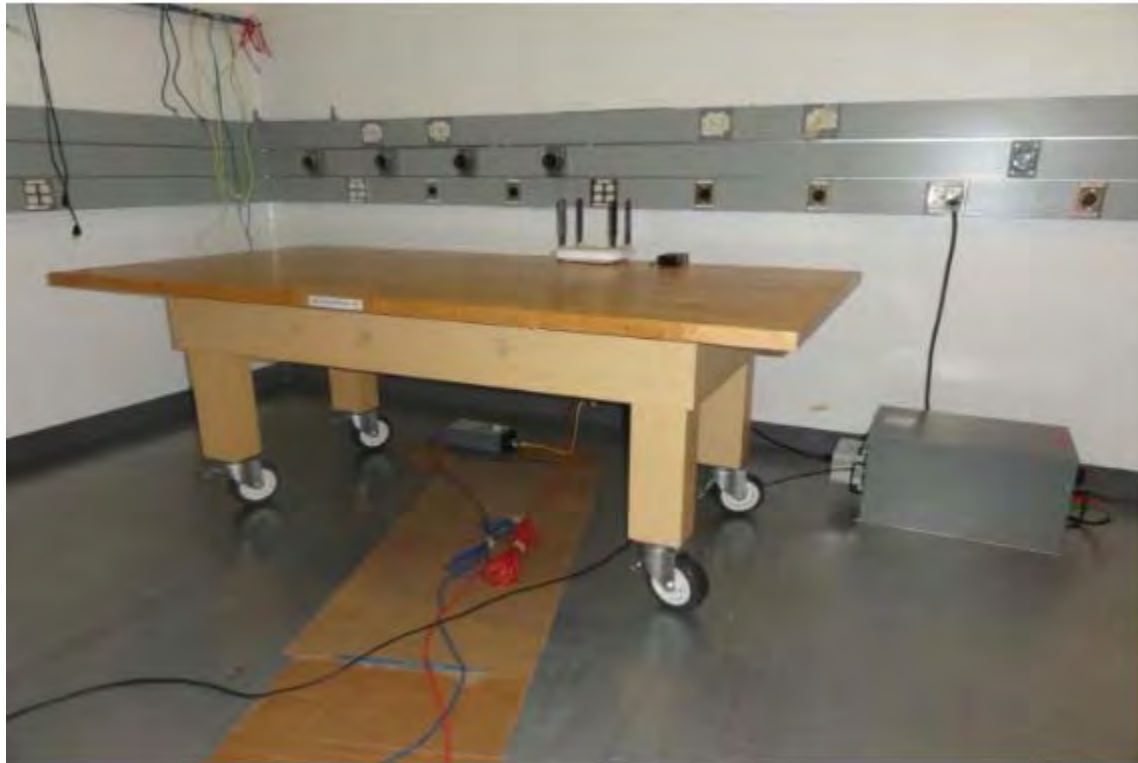
Test Setup for Conducted Measurements
