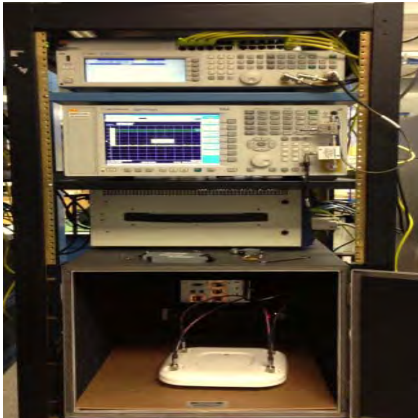
Test Setup for Conducted Measurements
