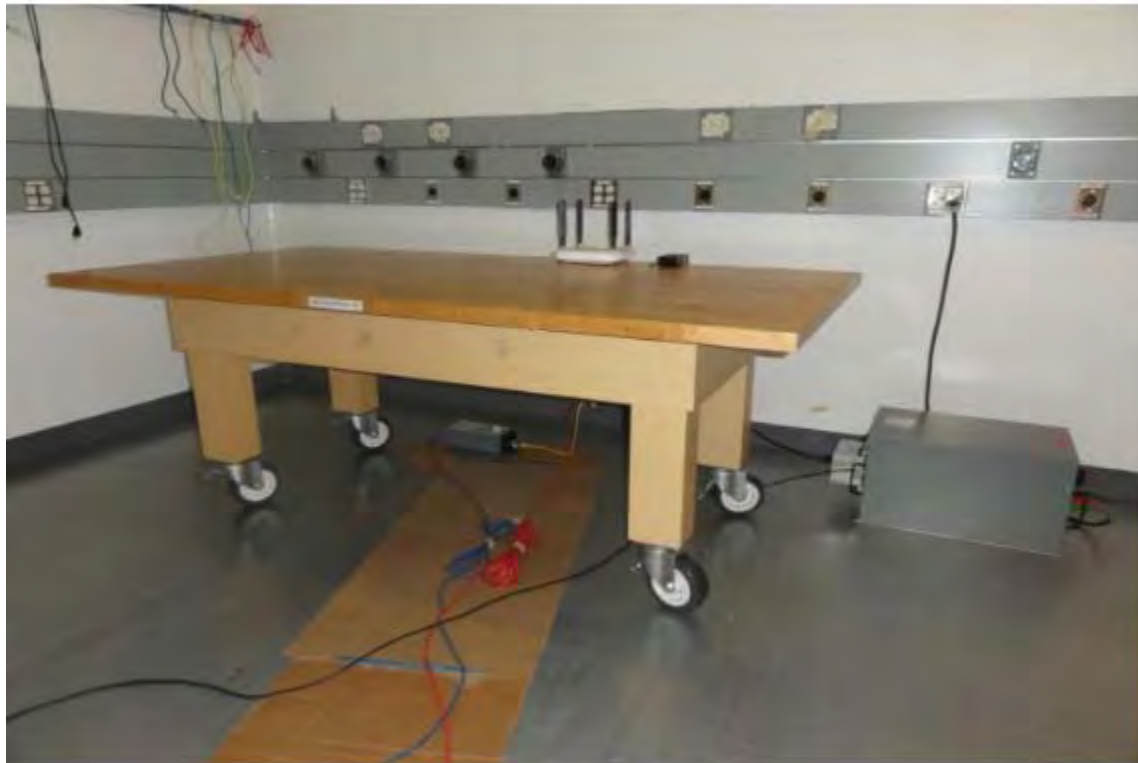
Test Setup for Conducted Measurements
