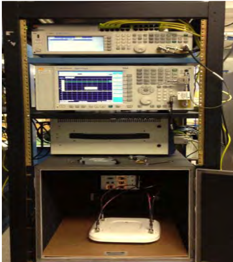
Test Setup for Conducted Measurements
