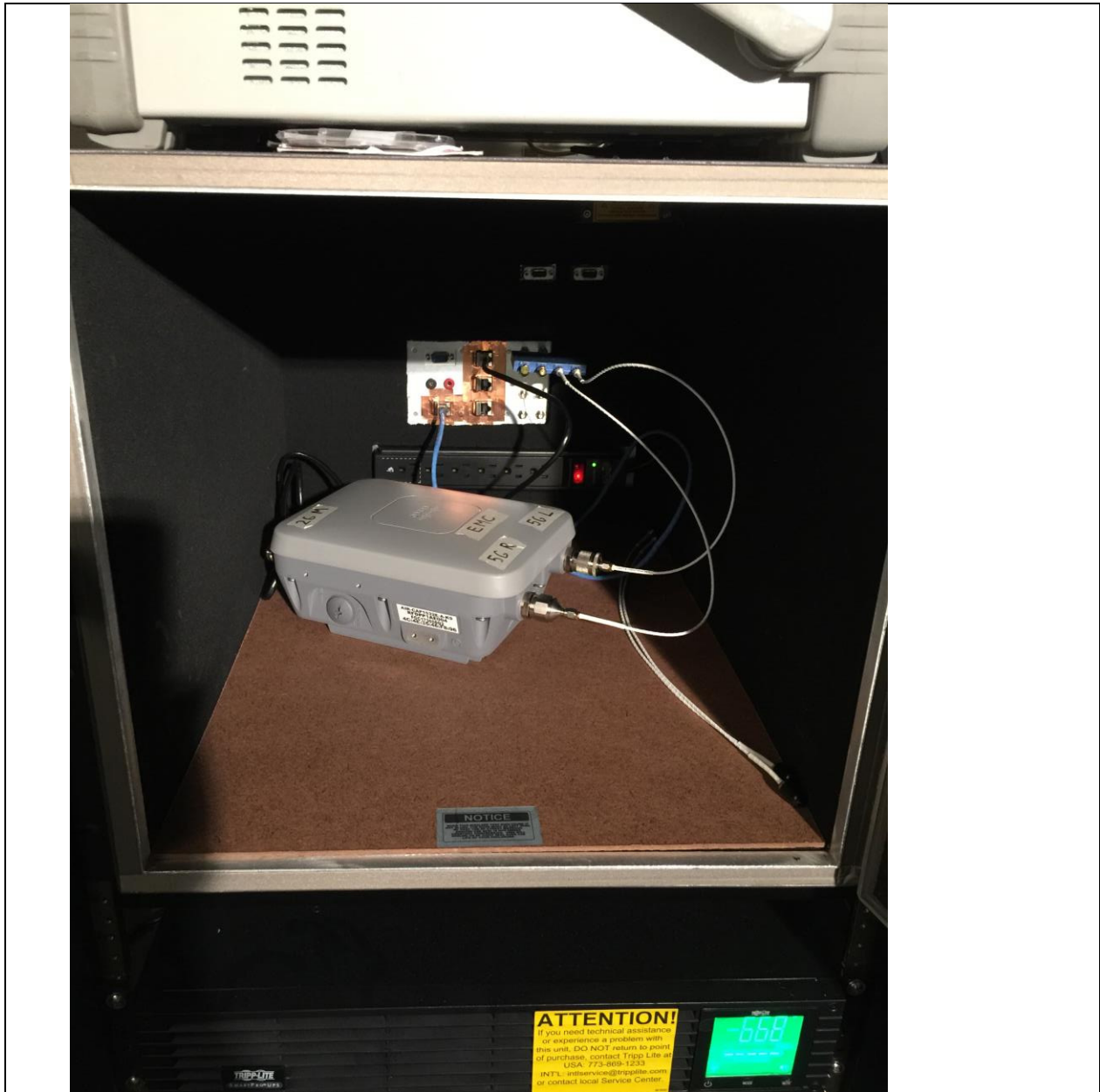
Title: AIR-CAP1532I-B-K9 Conducted Test Setup
