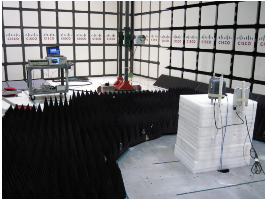
Radiated Test Setup 18-40GHz
